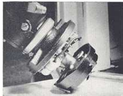
Fig. 13—Illustration of soldered-on timing stop.
