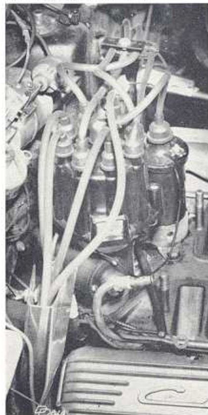
Fig. 11—Replacement ignition wiring.
